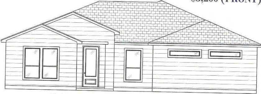
BASE ELEVATION - HARDI SIDING STANDARD
